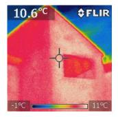
The 1990s house was the only one with cavity walls compliant with current building standards, and the cavity had been filled about ten years ago with fibre flock insulation. It had well fitting double-glazed windows, all its roofs were well insulated, and foil had been fixed behind radiators and inside the integral garage door. The entire house, even its conservatory, showed a more or less
