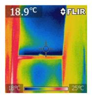
Then on to in North Kingston and the typical Victorian solid-walled semi, though again a house on which some retro-fitting had been undertaken in the form of double-glazed replica sash windows. These suited the style of the house and were much better than the originals, though still had a few of the leaky gaps
