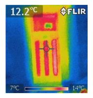
First was an extensively retro-fitted Edwardian house near the University – its solid walls externally insulated with phenolic foam cladding under new rendering, with some secondary double-glazing. These were working well, but the big surprise here was the original panelled Edwardian front door, with the thinner panels showing as markedly warmer than the rest of the house (see picture, left), betraying heat leaking out.
